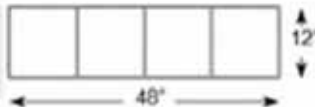
12" x 12" Slate Border FM-3300 S/O 12" x 48" (30.48 x 121.92 cm) Red A border of four 12" slate squares in a row Matching skin/touch-up wheel: Smooth Slate/TW-5 Joint size 1/4" wide, 1/2" deep
