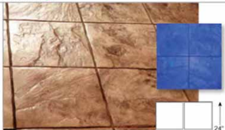
12" x 12" Slate, FM-3250 S/O 24" x 24" (60.96 x 60.96 cm) Blue Slate tiles laid in a parallel pattern Matching skin/touch-up wheel: Smooth Slate/TW-5 Joint size 1/4"-1/2" wide, 1/2" deep Stone size 12" square
